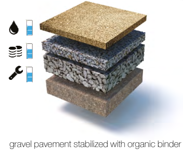
gravel pavement stabilized with organic binder
